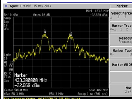
Screen snapshot of output power of the transmitter (around -23 dBm)
